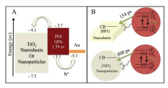
**Figure 2.** A) Schematic illustration of the energy level diagram of the PbS QDs/TiO<sub>2</sub> heterojunction solar cell. The positions of the energy levels were taken from ref. [12]. B) Illustration of the injection time from PbS QDs to 001 TiO<sub>2</sub> nanosheets and 101 TiO<sub>2</sub> nanoparticles. ps- picoseconds, CB-conduction band.
