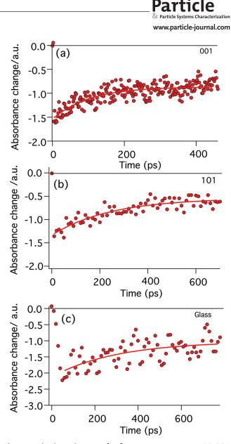
**Figure 4.** Bleaching dynamics for first excitonic transition  $(1S_h-1S_e)$  recorded at 870 nm following 520 nm excitation of PbS QD anchored on TiO<sub>2</sub> (001) nanosheets, (101) nanoparticles films and on top of a glass substrate. The absorbance bleach recovery is fitted by single exponential function. The solid lines represent the single exponential fitting. The fitting parameters are listed in Table 2.
