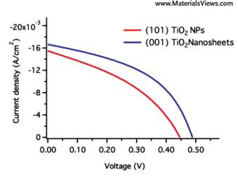
**Figure 5.** J–V curves of cells made of (001)  $TiO_2$  nanosheets and standard cells made of  $TiO_2$  NPs with dominantly exposed (101) facets.
