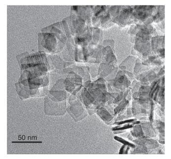
Figure 1. TEM image of 30 nm TiO<sub>2</sub> nanosheets used in this study.
